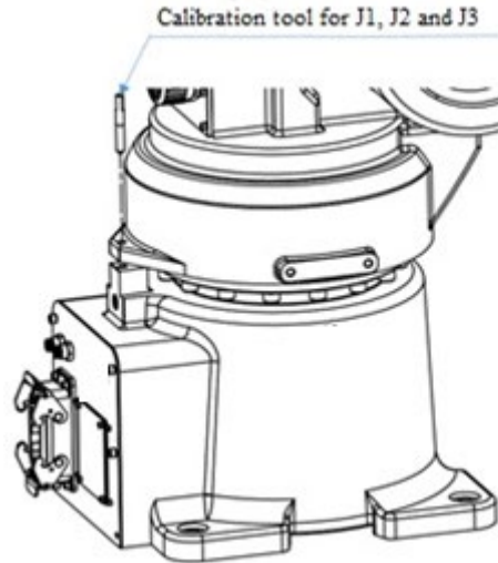
Figure 4-2 Illustration of J1-axis zero position setting
