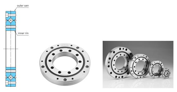
5. High rigidity with mounting holes (CRBE): Consisted of an inner ring and an outer ring with mounting holes. Because there are mounting holes, so it can be fixed directly and it is suitable for rotating of inner ring and outer ring both.
